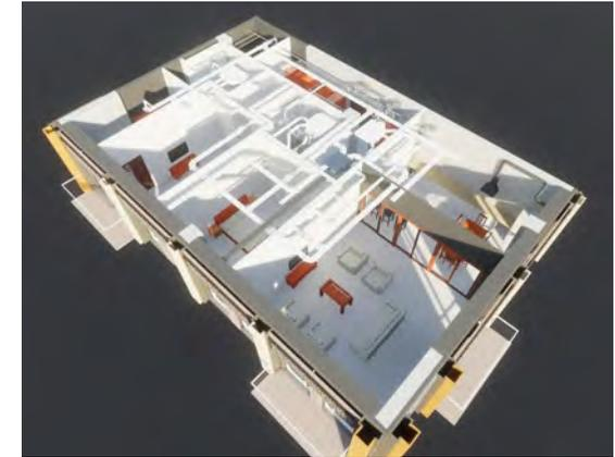
Option with central kitchen extract duct to the roof could undermine the flexibility principles, and but was chosen after weighting all options.
